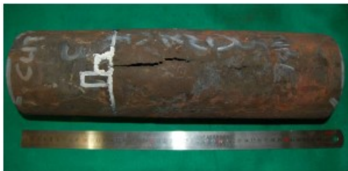
Figure 1: Macro-aspect of crack in bulged convection section pipe (Refinery "B")
